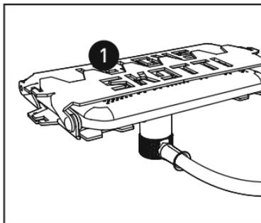
**1.** The booster unit (1) with burner is fitted with both the support surface (2 parts) and the feet, which must now be unfolded.
