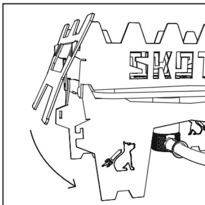
**6.** Now fold the side panel (3) down until it lies completely on the outer hook of the booster unit. Attach the second side panel (3) on the opposite side of the booster unit in the same way.
