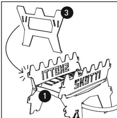
**4.** Continue with one of the two side parts (3), which is first hooked from above onto the outer hooks provided on the support surfaces on the booster unit (1).
