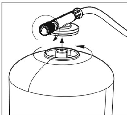
1. close the gas tap by turning it firmly to the right (☞) before connecting the gas cartridge.
