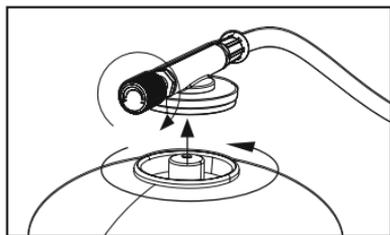
1. Close the gas tap by turning it firmly to the right (
