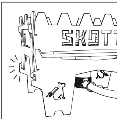
**7.** Now fold the feet slightly outwards so that you can slide them onto the hooks provided on the side panels (3). Then push the feet inwards again to lock the side parts (3) in place.
