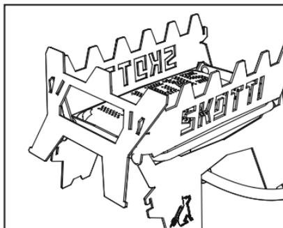
**5.** To have more contact surface, use the outer slots of the side parts during assembly. For smaller containers, you can use the inner slots.
