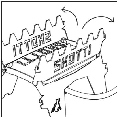
**3.** Then unfold the two top-mounted support surfaces to the left and right.
